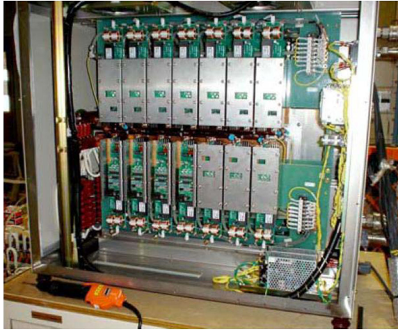
FIG. 28. A photograph of the SPS. There are seven MOSFETs in each arm.
