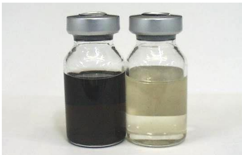
Figure 4. 3 Visual inspection on the stability of \text{LiPF}_4(\text{CF}_3)_2 electrolyte. The \text{LiPF}_4(\text{CF}_3)_2 electrolyte, i.e., 0.1 \text{ mol dm}^{-3} PC/DME (1/2 by volume) on the right, was stored for 3 years at room temperature. The \text{LiPF}_6 electrolyte on the left is also stored in the same condition in order to compared to the \text{LiPF}_4(\text{CF}_3)_2 electrolyte.
