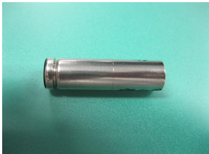
Figure 3. 1 A photograph of prototype 14500 lithium-ion battery. The battery is also called AA size battery, which is 14 mm in diameter and 50 mm height.
